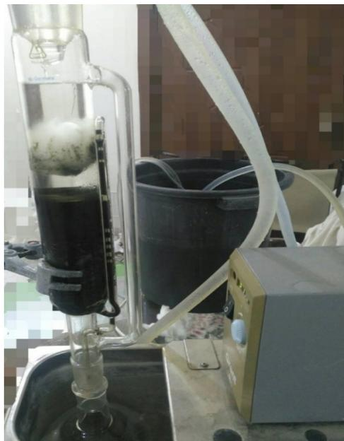
**Fig. 1 :** Oil extraction from algae using a Soxhlet extractor
