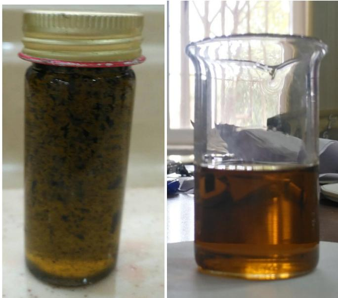
**C- Microalgae oil before filtration D- Microalgae oil after filtration****Fig. 5** : Extracted oil from *Scenedesmus ecornis* before and after filtration
