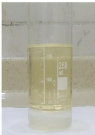
**Fig. 6 :** Biodiesel production from - *Scenedesmus ecornis* by transesterification process
